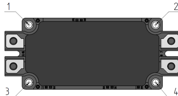
Figure 5: Screw positions in sequence
