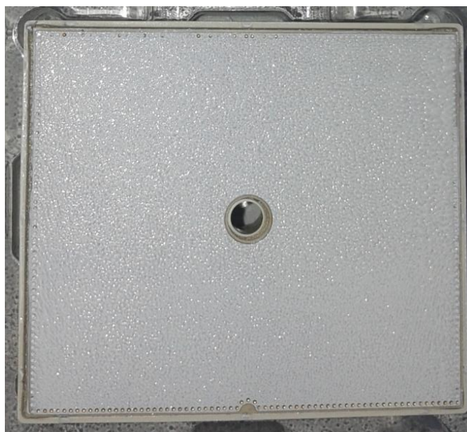
Figure 10 continuous layer of thermal paste
