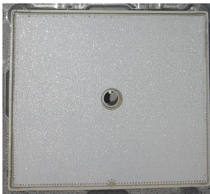
Figure 10 continuous layer of thermal paste
