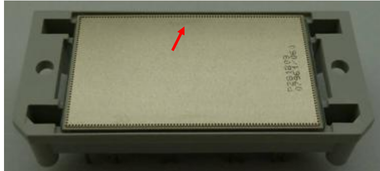
9. Figure: Discoloration of substrate
