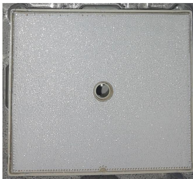
Figure 10: continuous layer of thermal paste
