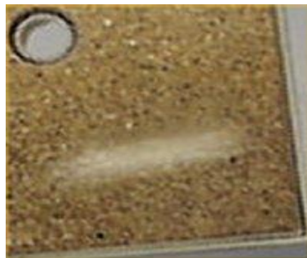
Figure 3: DCB's bottom surface after rework
