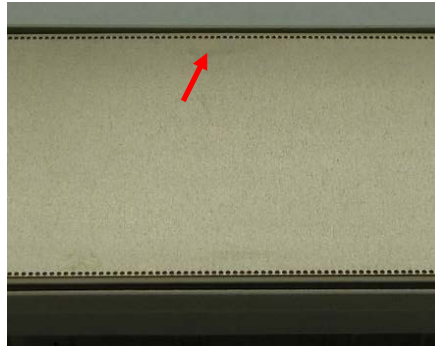
6. Figure: Discoloration of substrate
