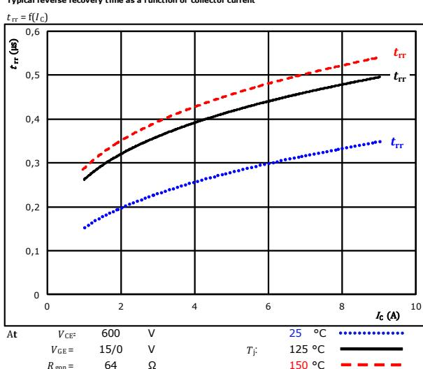
At  $V_{CE} = 600$  V       $T_j = 25$  °C       $I_C = 5$  A
