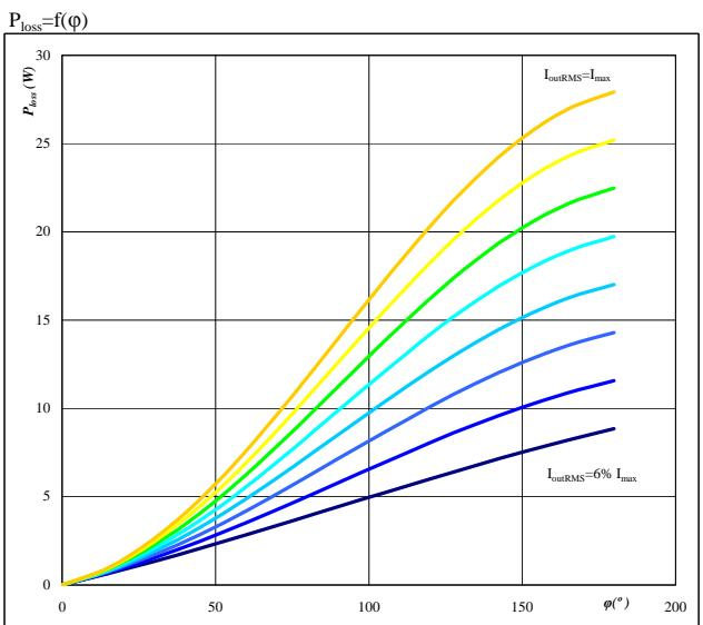
Conditions:  $T_j=125^\circ\text{C}$   $f_{sw}=16\text{ kHz}$
