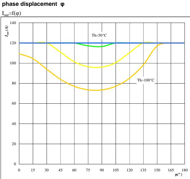
Conditions:  $T_j = 150/125^\circ\text{C}$        $f_{sw} = 16\text{ kHz}$
