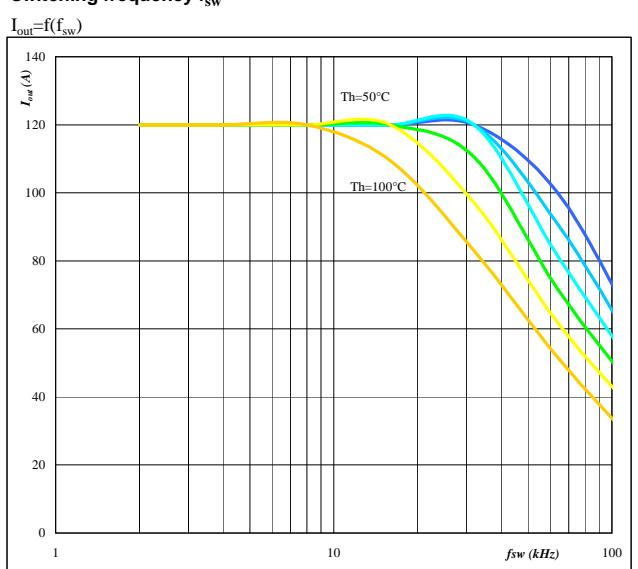
Conditions:  $T_j = 150/125^\circ\text{C}$        $\varphi = 0^\circ$
