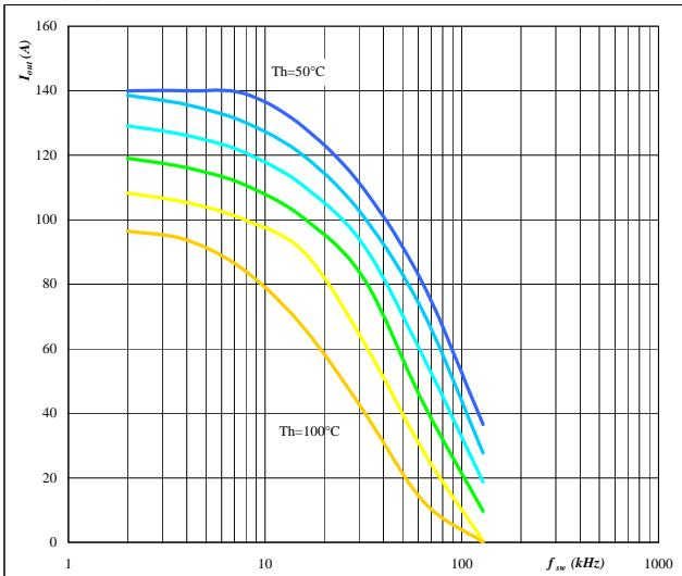
Conditions:  $T_j = 150/125 \text{ } ^\circ\text{C}$        $\varphi = 90^\circ$
