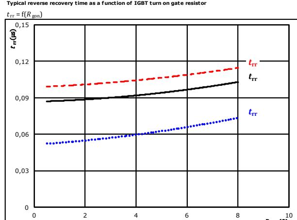
At  $V_{CE} = 350 \text{ V}$   $T_J = 25 \text{ } ^\circ\text{C}$   $I_C = 90 \text{ A}$
