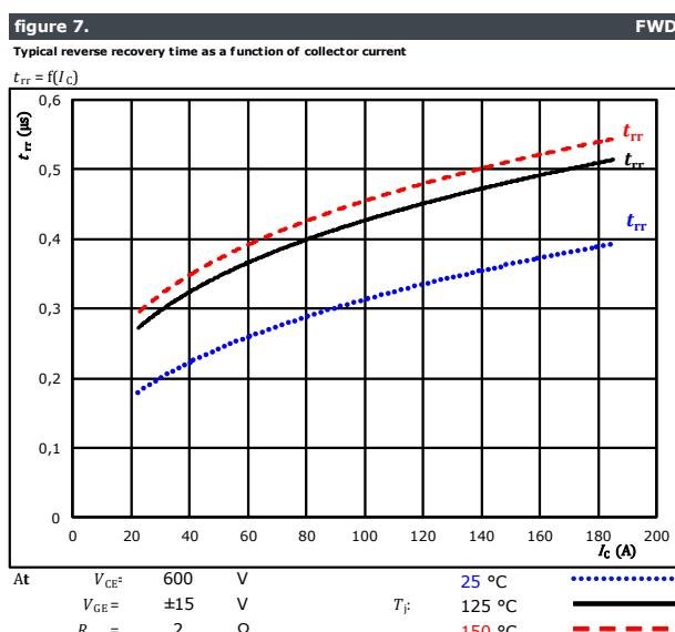
At  $V_{CE} = 600$  V       $T_j = 25$  °C       $t_{rr} = 0.28$  μs
