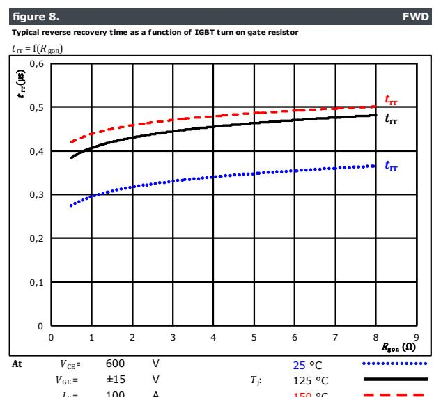
At  $V_{CE} = 600$  V       $T_j = 25$  °C       $t_{rr} = 0.42$  μs
