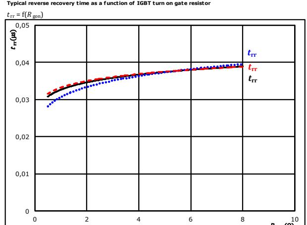
At  $V_{CE} = 600 \text{ V}$   $T_J = 25^\circ\text{C}$   $t_{rr} = \dots$
