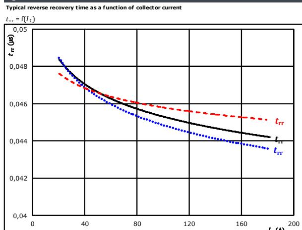
At  $V_{CE} = 600 \text{ V}$   $T_J = 25 \text{ } ^\circ\text{C}$   $R_{gon} = 2 \Omega$
