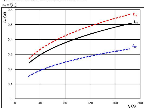
At  $V_{CE} = 600 \text{ V}$   $T_J = 25 \text{ } ^\circ\text{C}$   $R_{gon} = 2 \text{ } \Omega$
