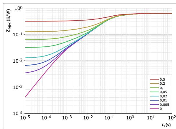
$$D = \frac{t_p}{T} \quad R_{th(j-s)} = \frac{t_p}{0,63} \quad K/W$$
