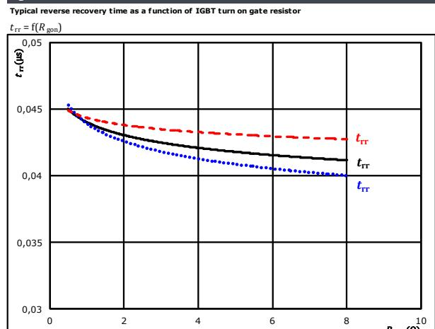
At  $V_{CE} = 600 \text{ V}$   $T_J = 25 \text{ } ^\circ\text{C}$   $R_{gon} = 2 \Omega$
