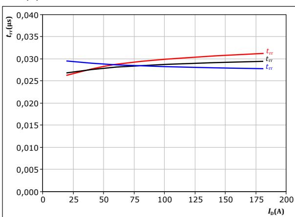
$$\begin{aligned} \text{At} \quad V_{DS} &= 600 \text{ V} \\ V_{GS} &= -2/15 \text{ V} \\ R_{gon} &= 2 \Omega \end{aligned}$$
