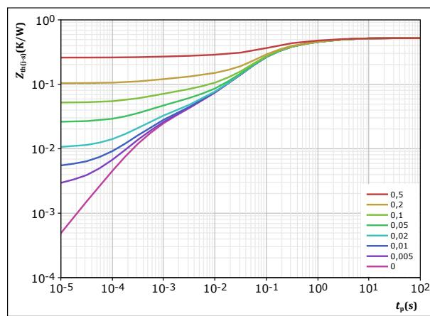
$$D = \frac{t_p}{\tau} \quad R_{th(f-s)} = \frac{t_p}{0,52} \quad K/W$$
