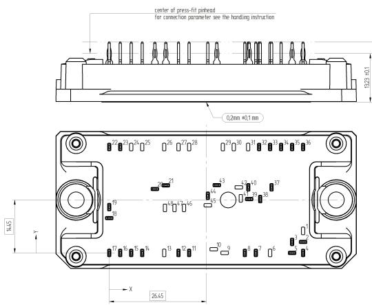
Tolerance of pinpositions: +/-0.1mm at the end of pins
