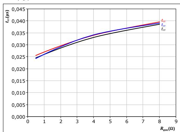
$$\begin{aligned} \text{At} \quad V_{DS} &= 600 \text{ V} \\ V_{GS} &= -2/15 \text{ V} \\ I_D &= 100 \text{ A} \end{aligned}$$
