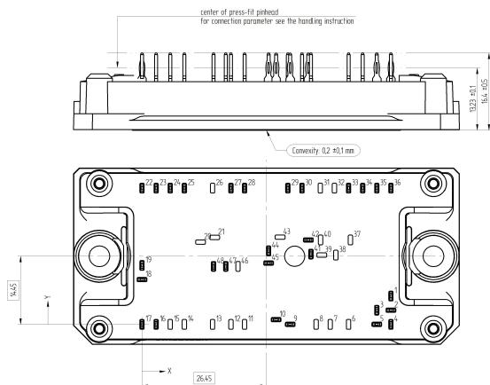
Tolerance of positions +/-0.1mm at the end of axis
