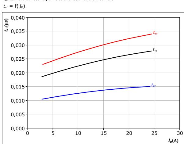
At  $V_{DS} = 400 \text{ V}$
