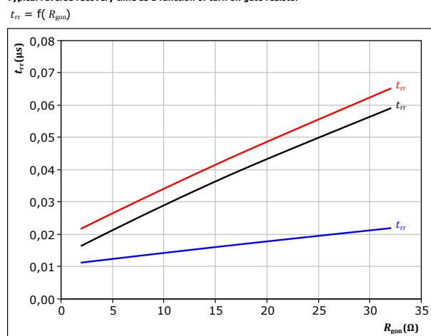
At  $V_{DS} = 400 \text{ V}$
