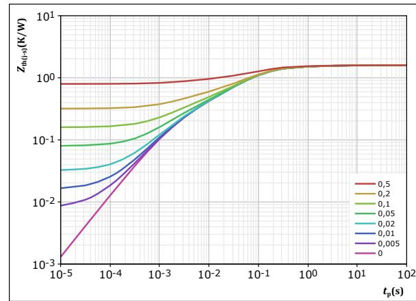
$$D = \frac{t_p / T}{1,594} \quad R_{th(t-s)} = \frac{1,594}{t_p / T} \text{ K/W}$$
