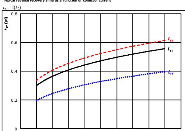
At  $V_{CE} = 600$  V       $T_j = 25$  °C       $R_{gon} = 32$  Ω
