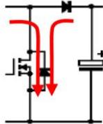
At switching-off the transistor the diode is commutated again and takes over the current.
