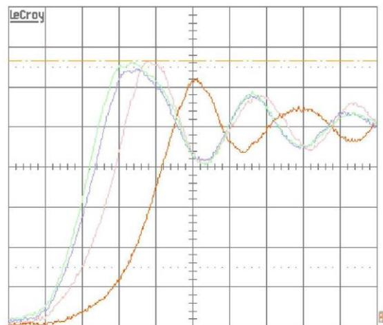
The figure shows a PFC Module without internal capacitor. The voltage overshoot reach 536V ( $V_{DC} = 400V$ )
