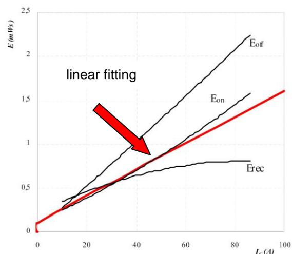
With  $I_n$  and  $U_n$  are the nominal current and output voltage where switching losses were measured and  $f_{\text{sw}}$  is a constant switching frequency:
