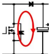
The current change rate and the parasitic inductance cause a voltage spike at the transistor according to:
