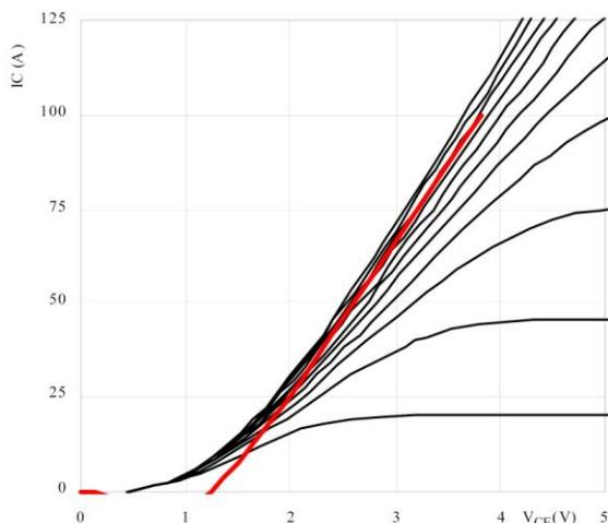
Therefore it is possible to describe the static characteristics with 2 parameters ( $U_{\text{th}}$ ,  $r_t$ ) and use them for the calculation of static losses.
