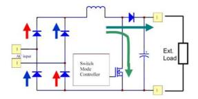
The input rectifier convert the AC voltage into a pulsed DC-voltage. The PFC-circuit boost both half waves to the DC-output voltage.
