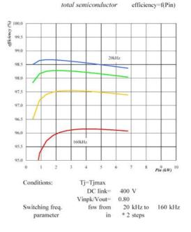
The efficiency of the semiconductors in a  $110V_{AC}$  system are: 94.8% (at  $V_{out} = 400V_{DC}$ ,  $P_{out} = 3kW$ ,  $f_{PWM} = 80kHz$ ). The efficiency advantage is ca. 1%.
