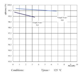
The efficiency of the semiconductors in the 230V system are: 97.4% (at  $V_{out} = 400V_{DC}$ ,  $P_{out} = 6kW$ ,  $f_{PWM} = 80kHz$ ). The efficiency advantage is ca. 0.5%.
