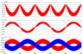
The results are deflating: All output signals of the PFC circuit are oscillating with the PWM frequency relative to the input.
