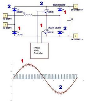
Here the current flow in the PFC-choke is bidirectional.
