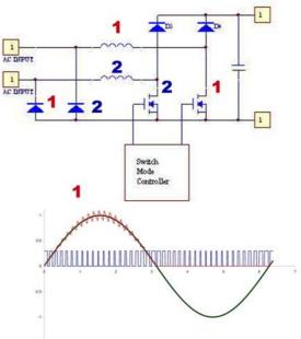
With this solution the output does not oscillate with high frequency relative to the AC-input or GND. The behavior is identical to the standard boost topology. But the losses of the input rectifiers used in the standard boost topology are cut into halves.
