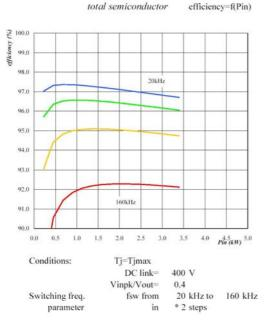
In both cases  $110V_{AC}$  and  $230V_{AC}$  input, the semiconductor losses are about 19% reduced compared with the standard boost topology.
