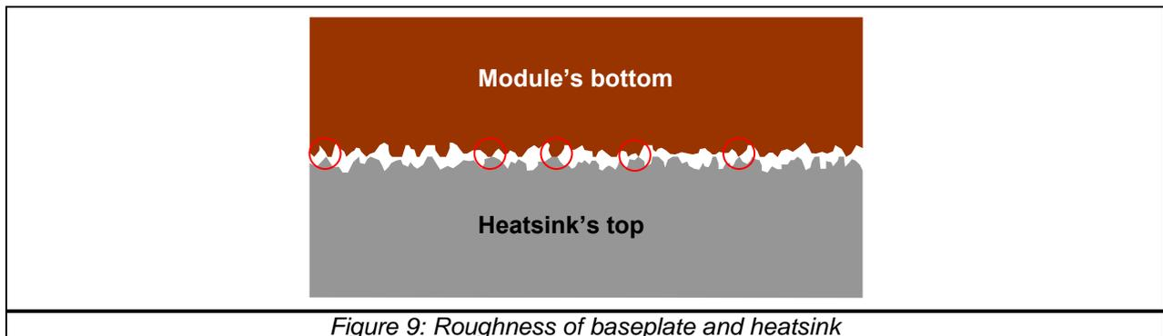
All areas that do not have metal to metal contact have to be filled with thermal interface material. It is obvious that the roughness of both parts is important for a good thermal contact. But also the size of the grains of a thermal compound is very important which is illustrated in the next figure.
