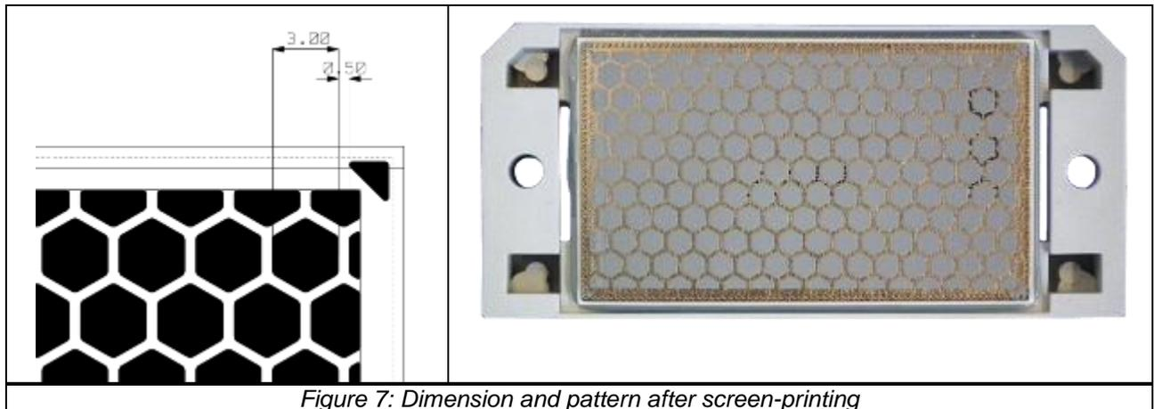
*Figure 7: Dimension and pattern after screen-printing*
