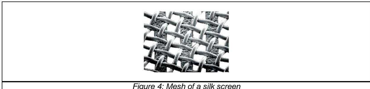
Silk screens allow applying a very thin layer which can be much thinner compared to stencils. Some thermal material remains in the meshes. Therefore a small variation of component from module to module is given as can be imagined when looking to Figure 4. The effort with these screens occurs in the adjustment above the module as well as in cleaning the screen afterwards. An application by machine with a constant pressure is recommended instead the application by hand.
