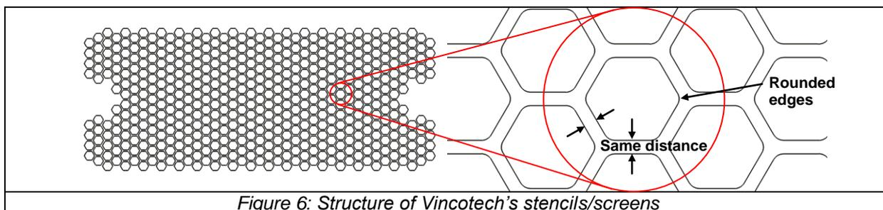
The amount of thermal compound can be varied with the thickness of the stainless steel stencils as well as with the thickness of webs. It is recommended to do a laser cutting of the stencil openings instead of a water-jet cut or instead of a chemical etching.
