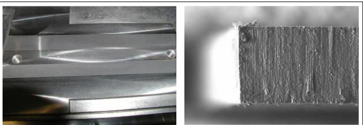
Figure 8a/b: Milled heatsink with grooves / magnification of roughness
