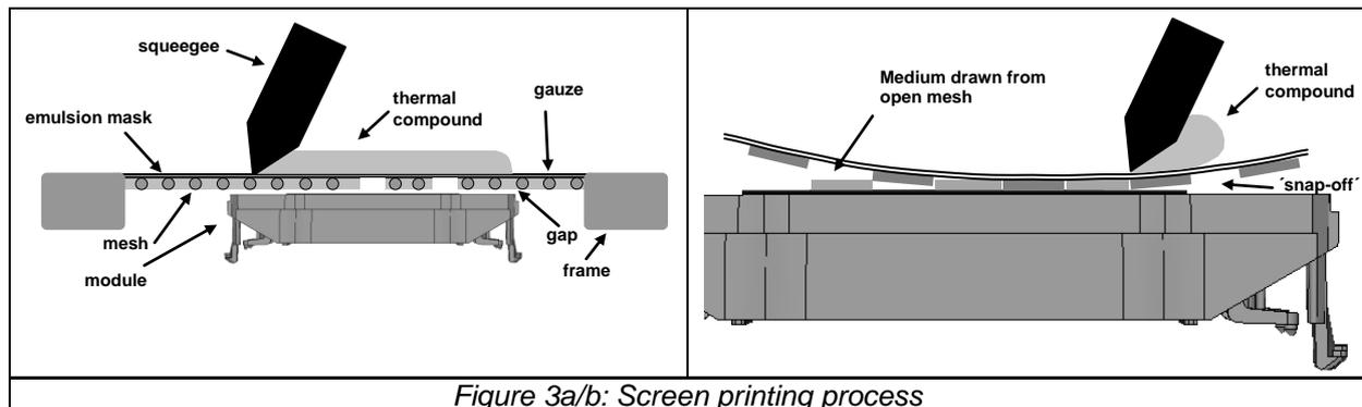
The squeegee blade presses the material into the open apertures of the screen, and then removes the rest as it passes across the aperture. The screen then peels away from the module behind the squeegee, leaving the material that was previously in the mesh aperture deposited on the module beneath.
