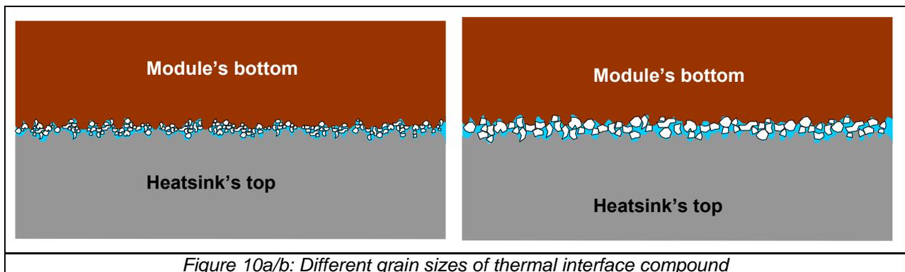
Figure 10a shows a thermal grease with small grain sizes where the sketch on the right hand shows thermal grease with big grain sizes. Blue areas depict the volatile content of the grease.
