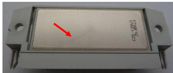
Figure 3: Discoloration of substrate
