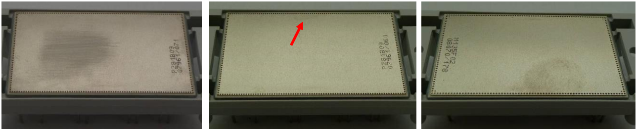
7. Figure (Left to right): Polished surface; Discoloration of substrate; Fingerprint on the surface
