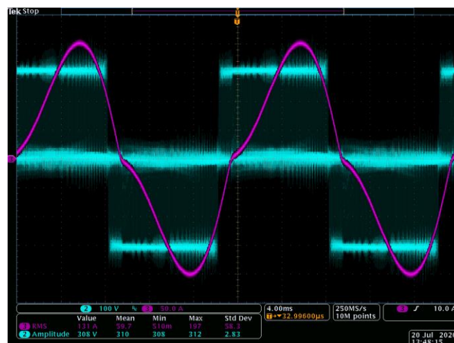
Figure 7: The output voltage (CH2) and the output current (CH3) in the EVA Board
