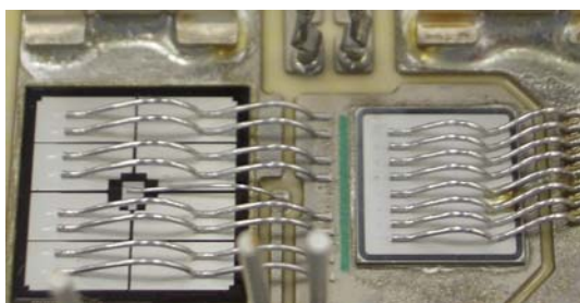
Fig. 3: Wire bonds as a source of stray inductance
