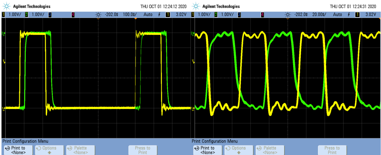
Figure 9 The delay between CLKI and the received CKO on the control card on 1,6 MHz and 16 MHz
